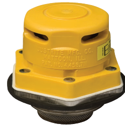
08006 Nonmetallic vertical vent, stainless steel flame arrester for chlorinated solvents DN50
